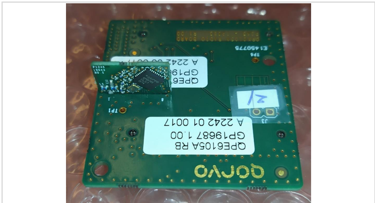
Figure 4: QPE6105A Module on Radio Adaptor Board
