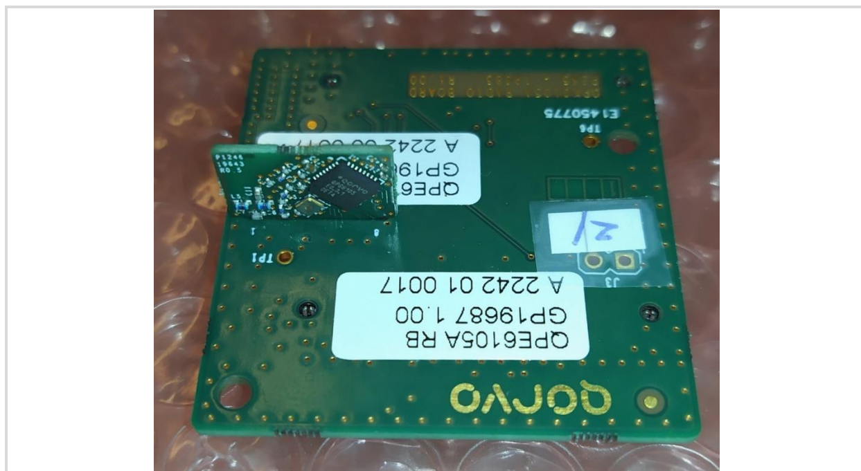
Figure 4: QPE6105A Module on Radio Adaptor Board
